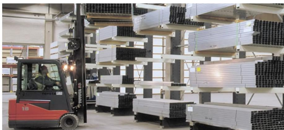
**Cantilever Racking, Pigeon-hole racks, Timber locker, A-Frame racks and racks for metal sheet are specially designed to store long goods and items of varying lengths.**
